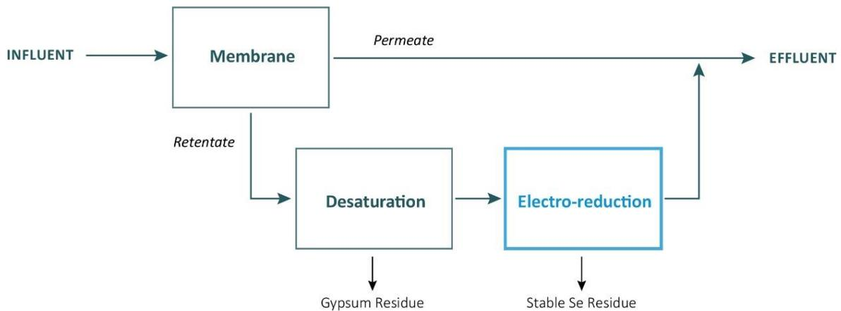
**Figure 6: Block Diagram of Treatment System for Simultaneous Sulphate and Selenium Removal**
