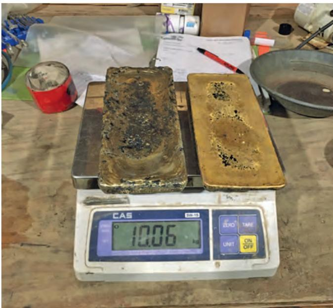
*Eleven test batches totalling around 2 t of a previously announced 5 t test sample from the 3 Aces gold project, in the Yukon, resulted in 93.17% recovery of contained gold, yielding 132.23 oz of gold doré, using EnviroLeach's non-cyanide, water-based, neutral pH treatment process*
