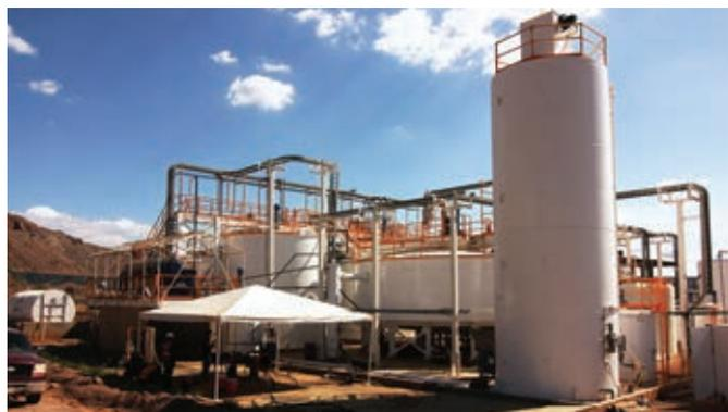
**From top to bottom:** Gypsum clarifier showing the clean overflow of the neutralized leach solution ready for use in the gold extraction circuit; Enclosed clarifier where copper precipitated from the leach solution is settled and filtrated to produce a high-grade copper concentrate with commercial value; Commissioning of a SART plant in Mexico to remove the metallurgical interference of copper in the orebody to improve gold extraction efficiency. CREDIT: BQE WATER
