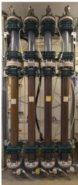
**Figure 3 Ion exchange columns in Selen-IX™ mobile pilot plant**
