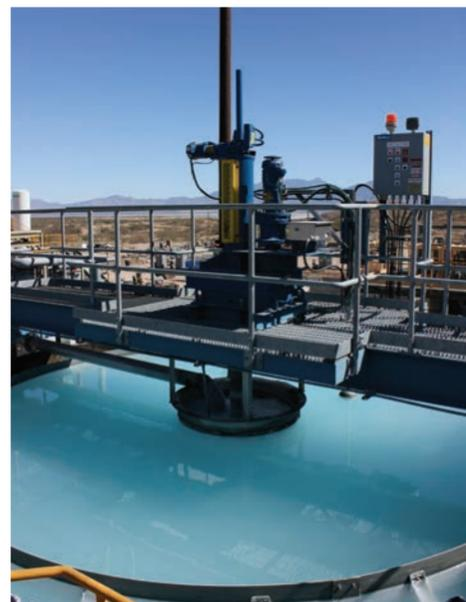
Top: BioteQ's Sulf-IX demonstration plant in Arizona was commissioned in the summer of 2012. Above: Clarifiers thicken and precipitate gypsum during resin regeneration. PHOTOS: BIOTEQ
